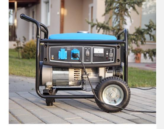
• For power outages, permanently installed stationary generators are better suited for providing backup power to the home. Even a properlyconnected portable generator can become overloaded. This may result in overheating or stressing the generator components, possibly leading to a generator failure.
